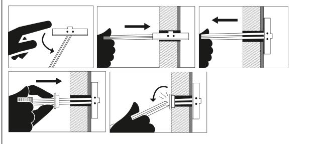
Insert the screw 3/16" X APPROPRIATE LENGTH into the hole and fasten the screw until the metal angle bracket is pulled snug against the wall.
