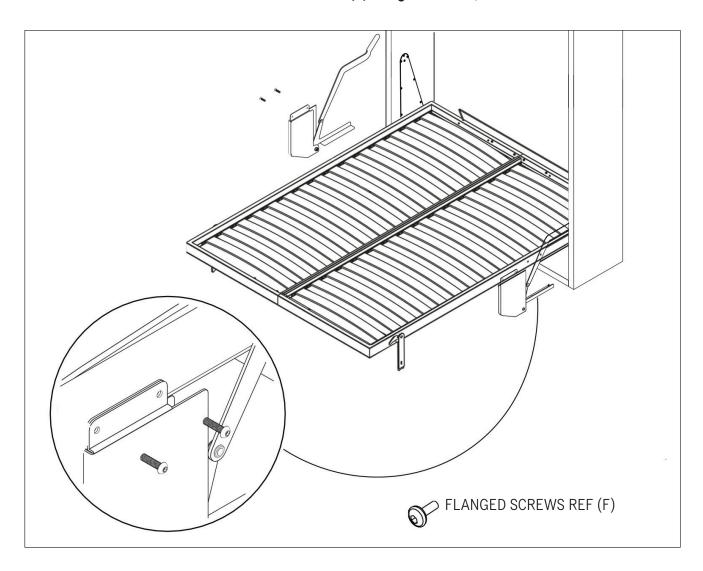
Bring the two bracket arms to the vertical panels, aligning the holes. Place the (G) conical washer between each panel and L-shaped bracket as shown in det. 11a - the conical washer's smallest diameter should face away from the panel so that it can fit within the L-shaped bracket. Secure the L-shaped brackets in place by screwing in a (G) flanged bolt into the brackets and panels, as shown in det. 11b.
