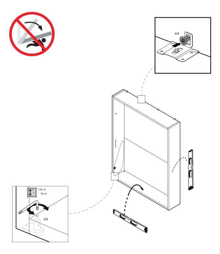
After the unit is level and plumb it should be securely attached to the wall using the metal angle mounting brackets as shown in the images below. A proper wall anchor suitable for the wall's construction must be selected by the contractor or installer.
