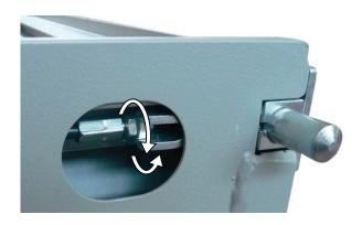
**3** Once the cable is adjusted correctly, and the levers are functioning properly, Tighten the lock nuts.
