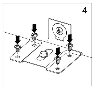
For 1/2" and 5/8" thick sheetrock it is recommended to use (4) 3/16 strap toggles.
