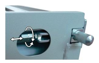
**2**. To shorten the pin, turn the adjustment screw clockwise. To lengthen the pin, turn the adjuster anticlockwise.
