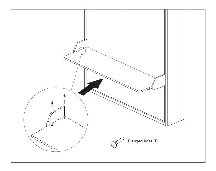
Insert 4 (I) flanged bolts into the holes on the desk, making sure that they pass through both the desk and the bracket arms (det. 13a). Once the bolts have been inserted, attach 4 (J) nuts, as shown in det. 13b. Tighten the hardware so that the nut head sits within the hole of the desk.
