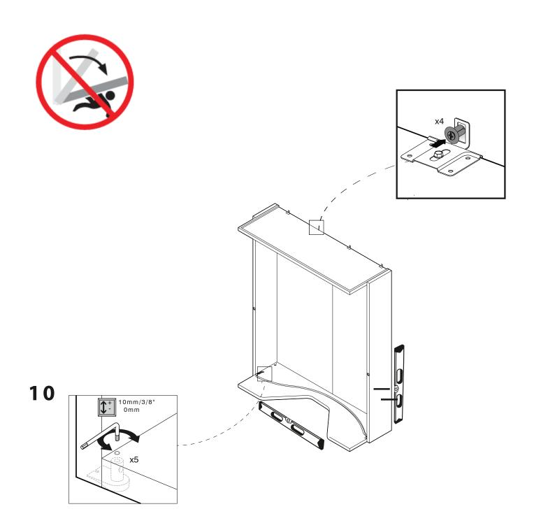
After the unit is level and plumb it must be securely attached to the wall using the metal angle mounting brackets as shown in the images below. A proper wall anchor suitable for the wall's construction must be selected by the contractor or installer.
