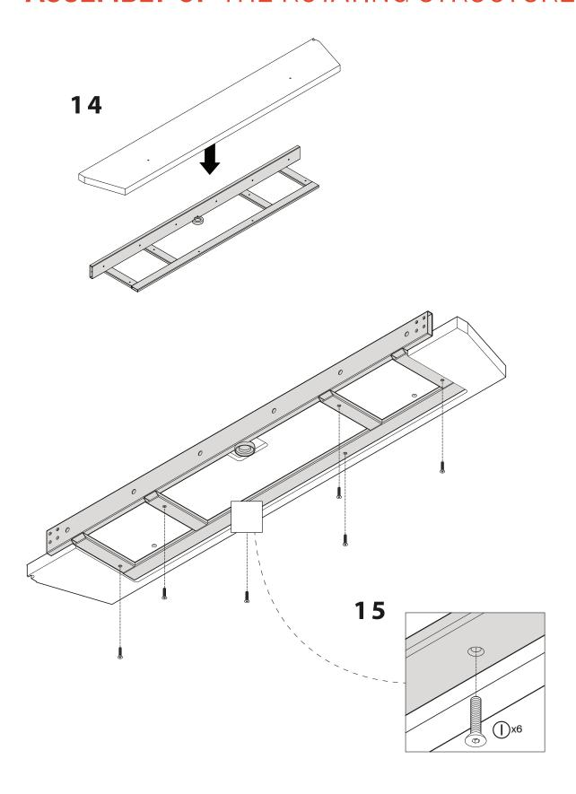
**Note:** Carefully drive bolts "I" into the bottom of the shelf. Do not overtighten as this may cause damage.
