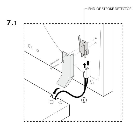
Connect the cable to the end of stroke detector
