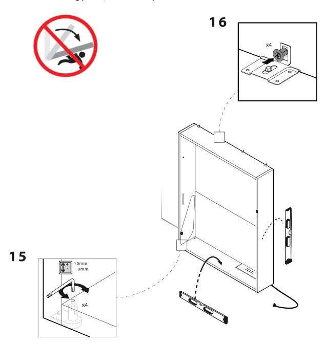
After the unit is level and plumb it must be securely attached to the wall using the metal angle mounting brackets as shown in the images below. A proper wall anchor suitable for the wall's construction must be selected by the contractor or installer.
